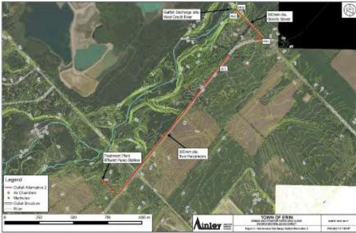
Figure 3 – Wastewater Effluent Discharge Outfall Alternative 2
