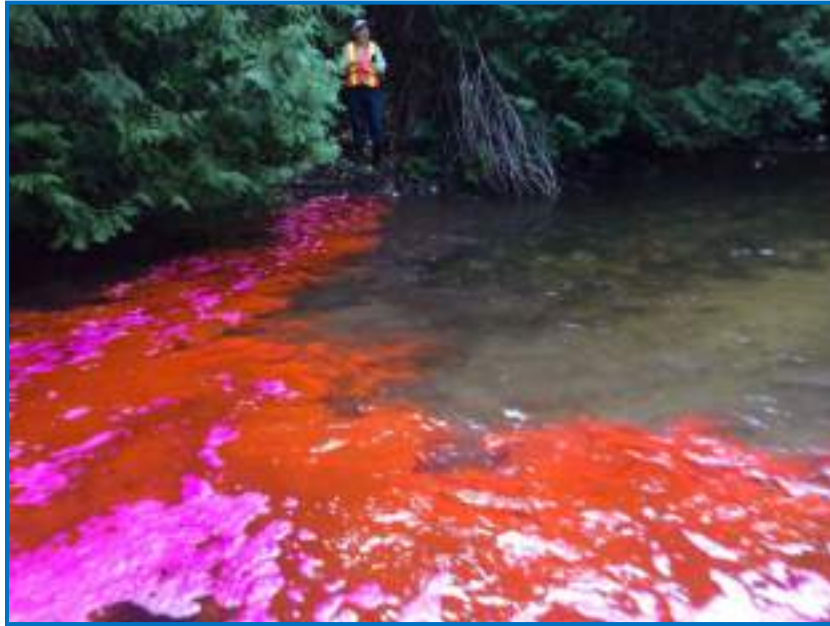
Photograph 2. Rhodamine WT Dye Plume Approximately 10 seconds after Slug (Instantaneous) Injection
