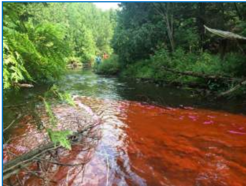
Photograph 3. Rhodamine WT Dye Plume Approximately 1 minute after Slug (Instantaneous) Injection.
