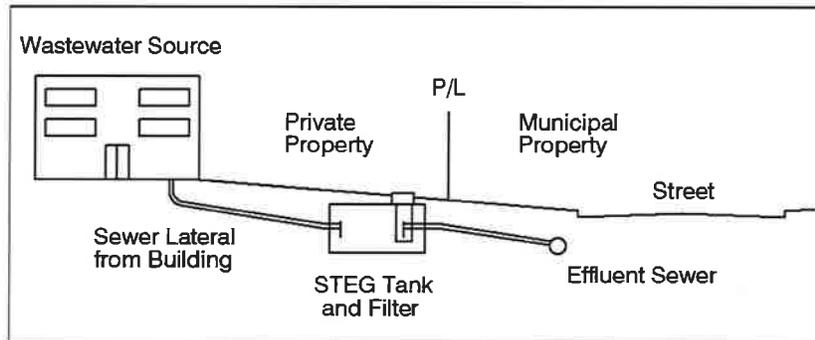
As a collection system, effluent sewers are used to convey effluent from multiple sources to a central location where it can be treated. STEP and STEG configurations can be combined within a given collection system. In a STEG system, each source or group of sources has a watertight septic tank with an effluent screen and an access riser. Effluent flows out of the tank and into a collection sewer by gravity (Water Environment Research Foundation, 2014).
