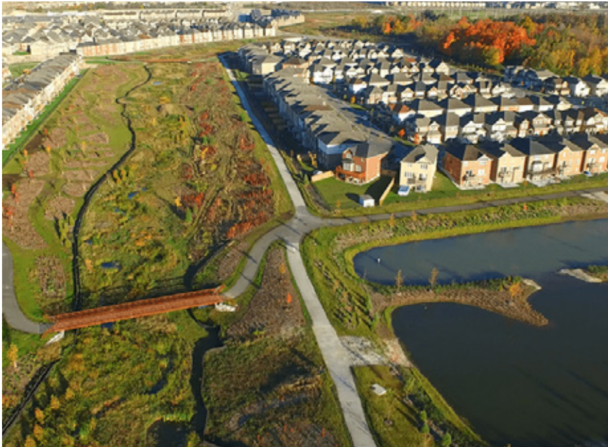
Figure 3.22: Image example of a SWM pond and residential neighbourhood adjacent to a Greenlands feature.
