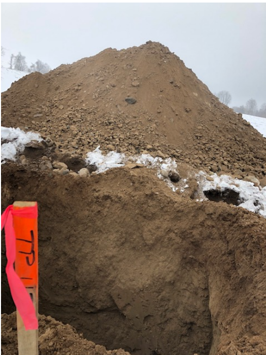
Photograph 16- View of excavated soils from TP 112. After 4.5 hours, test pit was dry and no cave-in observed.
