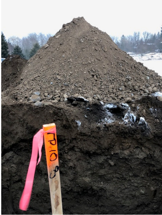
Photograph 9- View of excavated soils for TP108. Test pit was dry upon completion.
