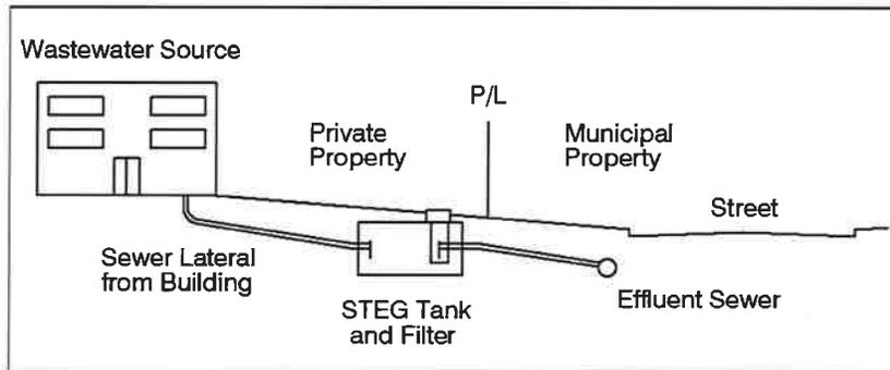
As a collection system, effluent sewers are used to convey effluent from multiple sources to a central location where it can be treated. STEP and STEG configurations can be combined within a given collection system. In a STEG system, each source or group of sources has a watertight septic tank with an effluent screen and an access riser. Effluent flows out of the tank and into a collection sewer by gravity (Water Environment Research Foundation, 2014).
