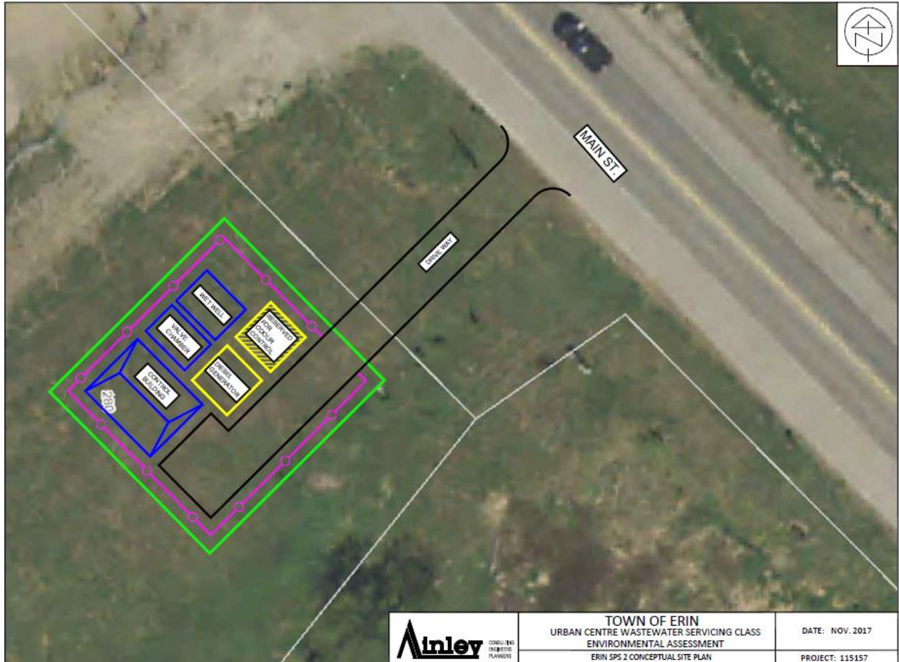
Figure 10 – E-SPS 2 Conceptual Site Plan
