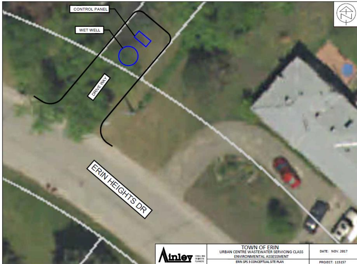
Figure 13 – E-SPS 3 Conceptual Site Plan
