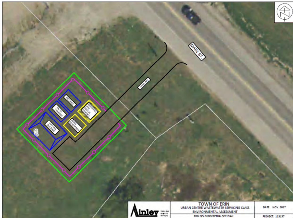
Figure 21 – E-SPS 2 Conceptual Site Plan
