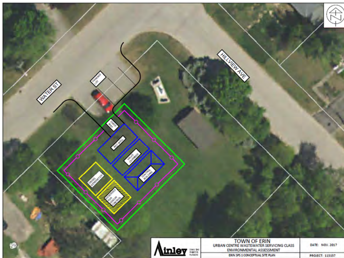
Figure 19 – E-SPS 1 Conceptual Site Plan
