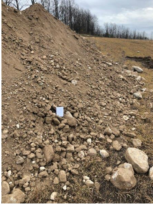
Photograph 5- Excavated soils from TP5. Note large boulders in soil pile.
